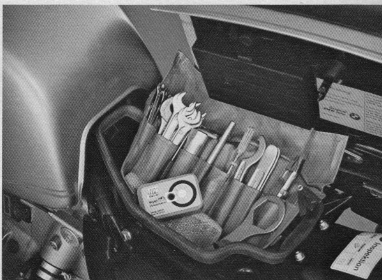
Flip up the locking seat and you'll find motorcycling's most complete tool roll—including a tire repair kit. Not shown: a tire pump. Tray is removable.
